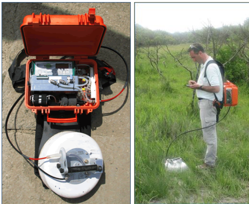
Fig. 5.3 Portable diffuse flux meter for carbon dioxide and methane (WEST Systems)
