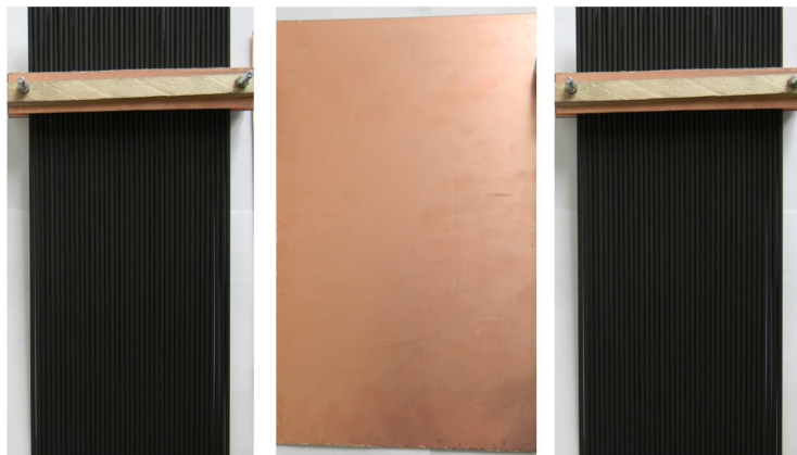
Figure 6.4. The plan parallel electrodes of the electrochemical reactor.
