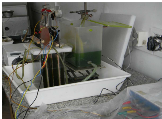
Figure 6.3. Schematic illustration of the lab-scale copper recovery equipment.
