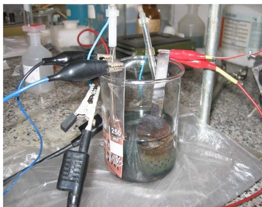
Figure 6.1. ER for Cu recovery from WPCBs by anodic dissolution and cathodic electrodeposition.
