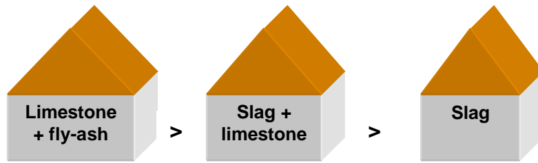
Fig. 7.3.2 – Indoor radon concentration based on addition types used in cements
