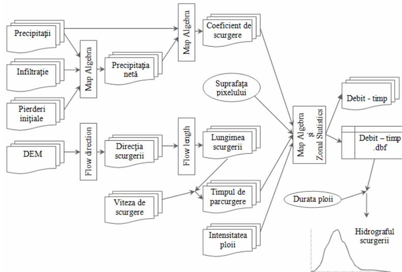
**Fig. 8.2.** GIS flood modeling algorithm schema taking in account soil water infiltration
