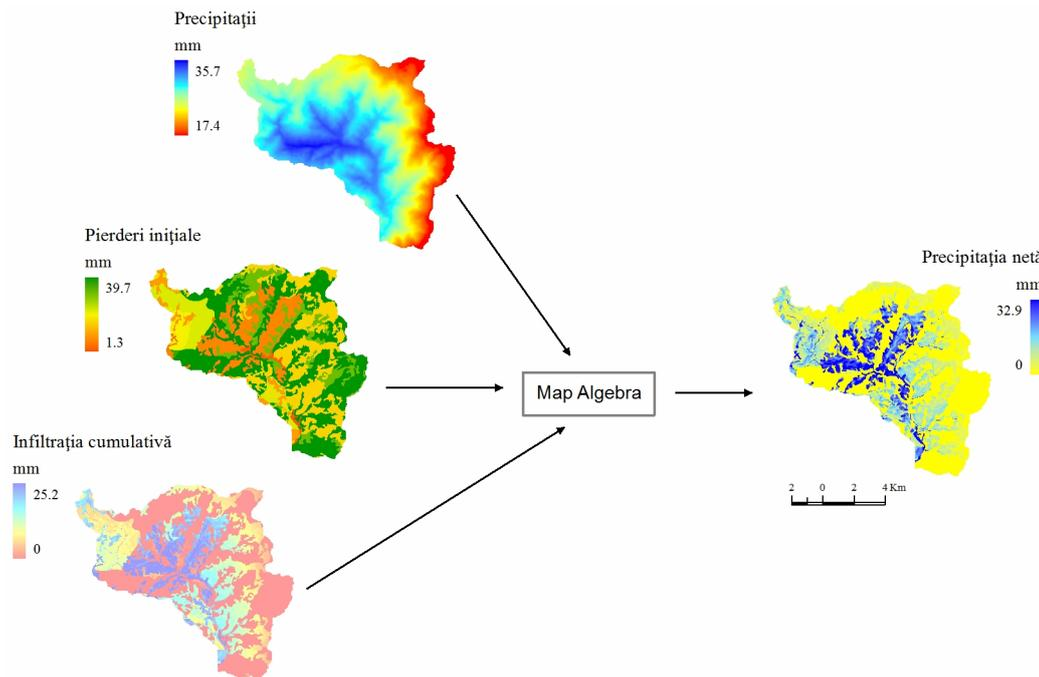
Fig. 8.3. Spatialization schematization algorithm of net rainfall using SCS-CN method
