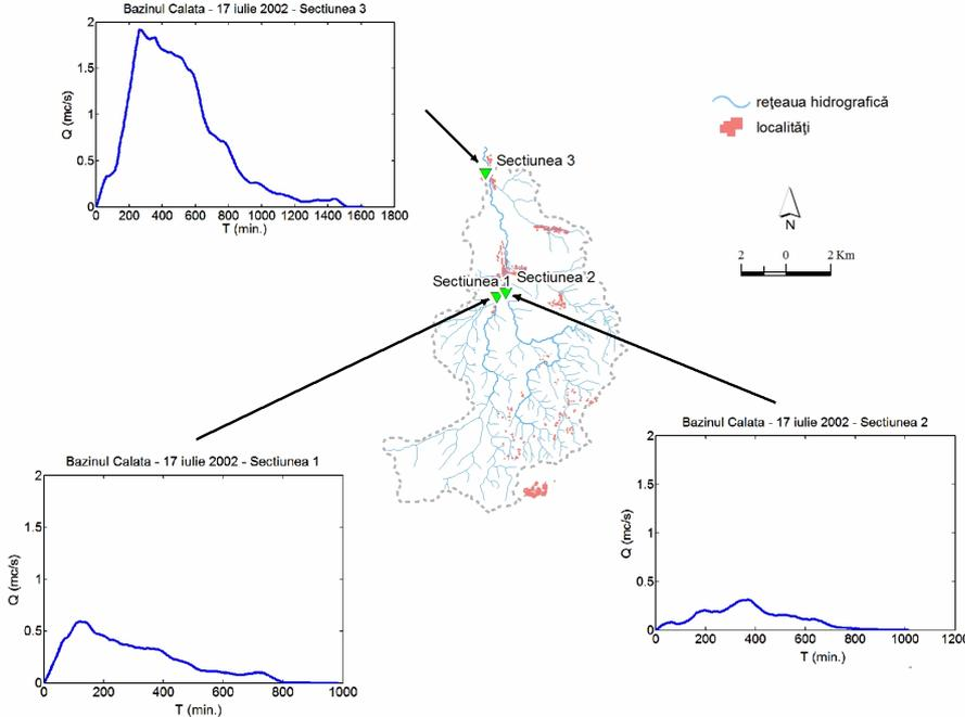
**Fig. 8.6.** Călata Watershed. Flow hydrograph generated by rain on the day of July 17, 2002
