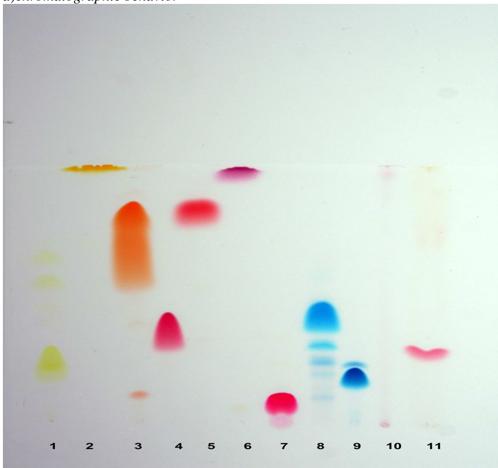
Fig.9. Chromatogram for: 1-quinoline yellow, 2-tartrazine, 3-sunset yellow FCF, 4-azorubine, 5-ponceau 4R, 6-erythrosine, 7-amaranth, 8-brilliant blue, 9-V patent blue, 10-carmine, 11-extract of soft drinks. Stationary phase – C 18 chemically modified diatomaceous earth, mobile phase: absolute ethanol – K 2 SO 4 0,5% in water (40:60, v/v) [313].
