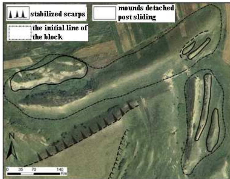
Fig. 6. The way in which the mounds from Boju have formed.
