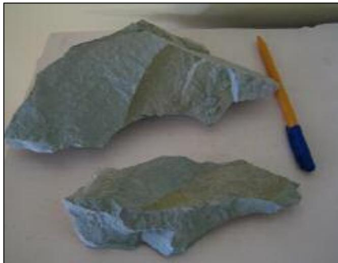
Fig. 4.3. Samples of volcanic zeolitic tuff from quarry of Valea Morii (sampling and photo: Irina Smical)
