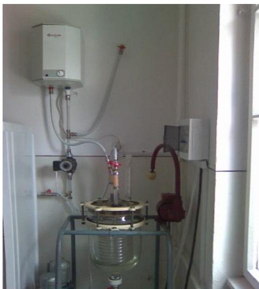
Figure 3.1 Installation for hydroxyapatite preparation.
