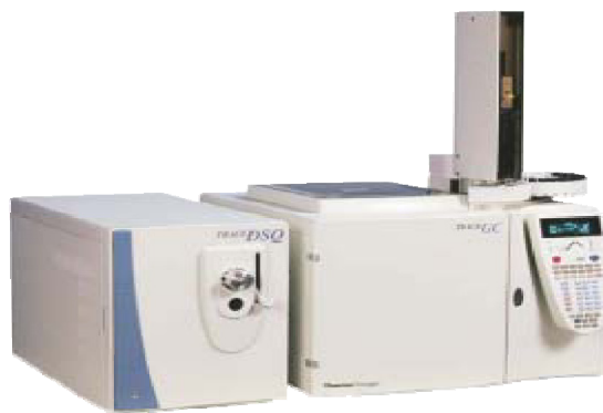
Figure 1.2. Trace DSQ ThermoFinnigan coupled with Trace GC- system equipped with autosampler
