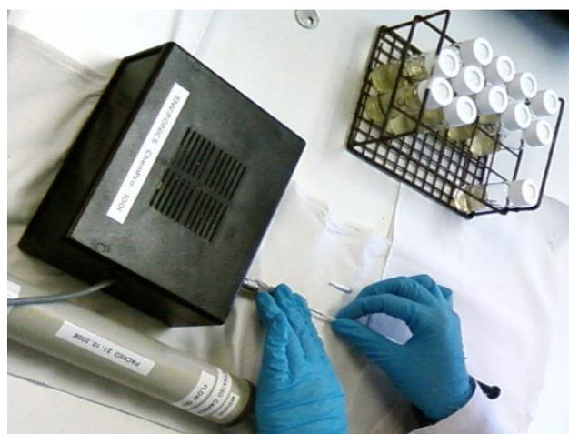
**Figure 11. Injection of samples in ChemPro100i IMS device**
