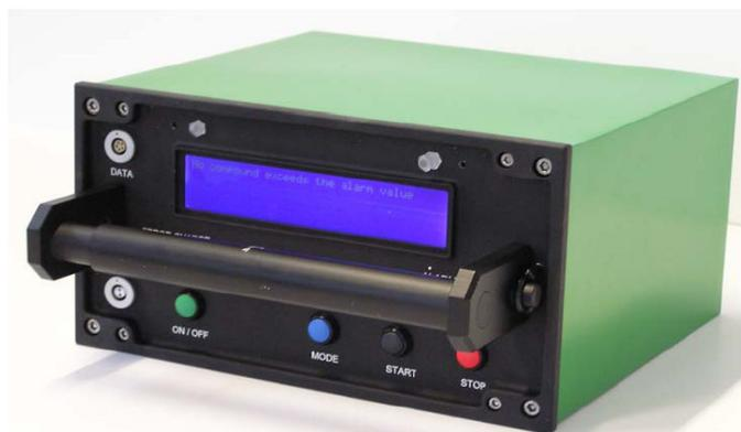
**Figure 4. Ion mobility spectrometer IMS-MINI (I.U.T. GmbH Berlin)**
