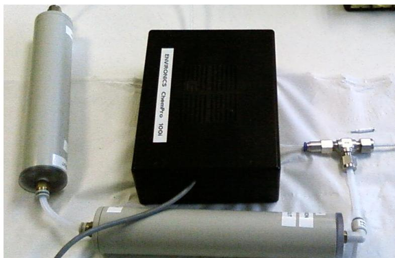
**Figure 6. Snapshot of Ion Mobility Spectrometer with transversal electric field (EnviroNics IMS)**
