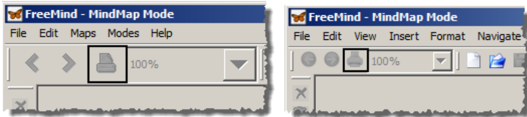
Figure 4.4: Icon changes can lead to widgets not being adequately matched
